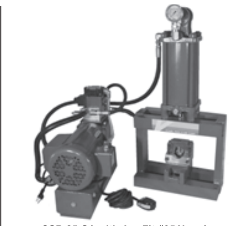
CSP-25-SA with Arc-Fit #35 Housing, #201A Punch Press Adaptor & Assembly
