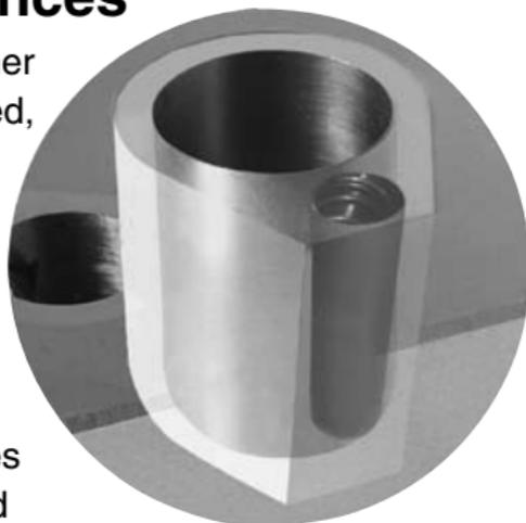
receptacle for the punch. One side of the piece (the flat side) is cut at an 8° angle to create a wedge shape. The hole in the retainer is wire cut to create a snug fit. (See cutaway.)
