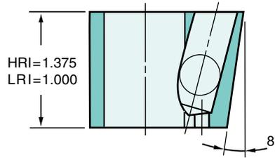
The shape shown above can be easily cut using wire EDM to assure a proper fit. The insert (utilizing both the straight and 8° angled sides) fits securely and is designed to clear the retainer by a small amount, making assembly and disassembly easier.
