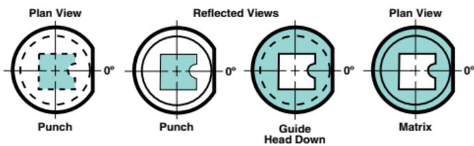
The reflected view is used for punches and guides. It is the view as seen in a mirror held below a punch or guide in its operating position. It is the same as a plan view from the head end, in which the point shape is shown dotted. A reflected view is shown with solid lines.
