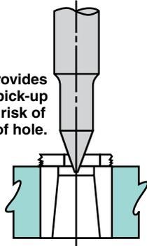
Greater positioning—moves stock farther than conventional pilots.
