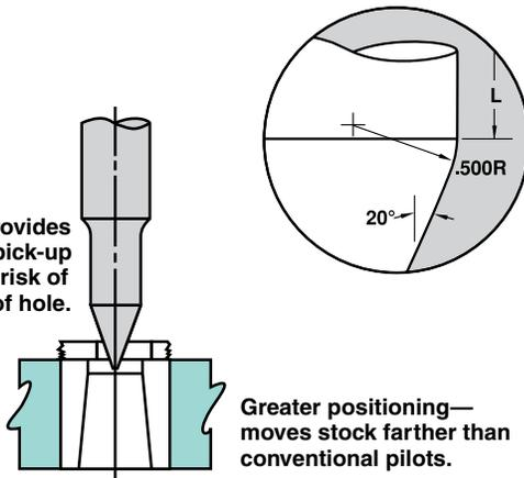
Greater positioning—moves stock farther than conventional pilots.
