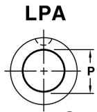
Geometry provides smoother pick-up without risk of distortion of hole.
